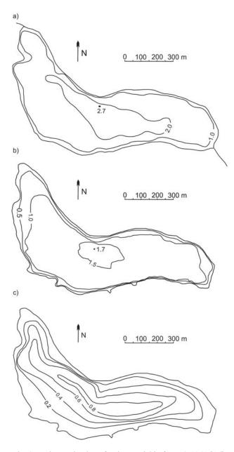
Fig. 3. Bathymetric plan of Lake Tomickie from a) 1961 [16], b) 2008 and shallowing of Lake Tomickie, c) between 1961 and 2008.
