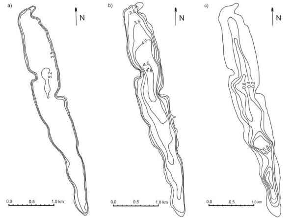
Fig. 2. Bathymetric plan of Lake Niepruszewskie from a) 1961 [15], b) 2008 and shallowing of Lake Niepruszewskie c) between 1961 and 2008.
